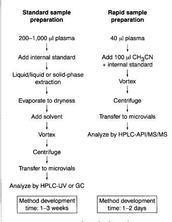
Figure 1. Comparison of standard sample preparation versus rapid sample preparation.
