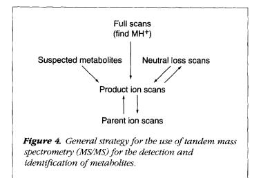
to a precursor ion scan except that the characteristic fragment selected is a neutral species rather than an ionic species. Conjugated species such as glutathione or sulfate give characteristic neutral losses when fragmented in a mass spectrometer; therefore, these metabolites can often be detected with a neutral loss scan.
