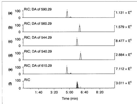
**Figure 7.** Mass chromatograms from the HPLC-API/MS/MS analysis of an extract of a rat plasma sample spiked with four drugs (traces a, b, d, e) at a level of 50 ng/ml each, plus the internal standard (c); trace f is the reconstructed ion chromatogram (RIC); DA = daughter ion.
